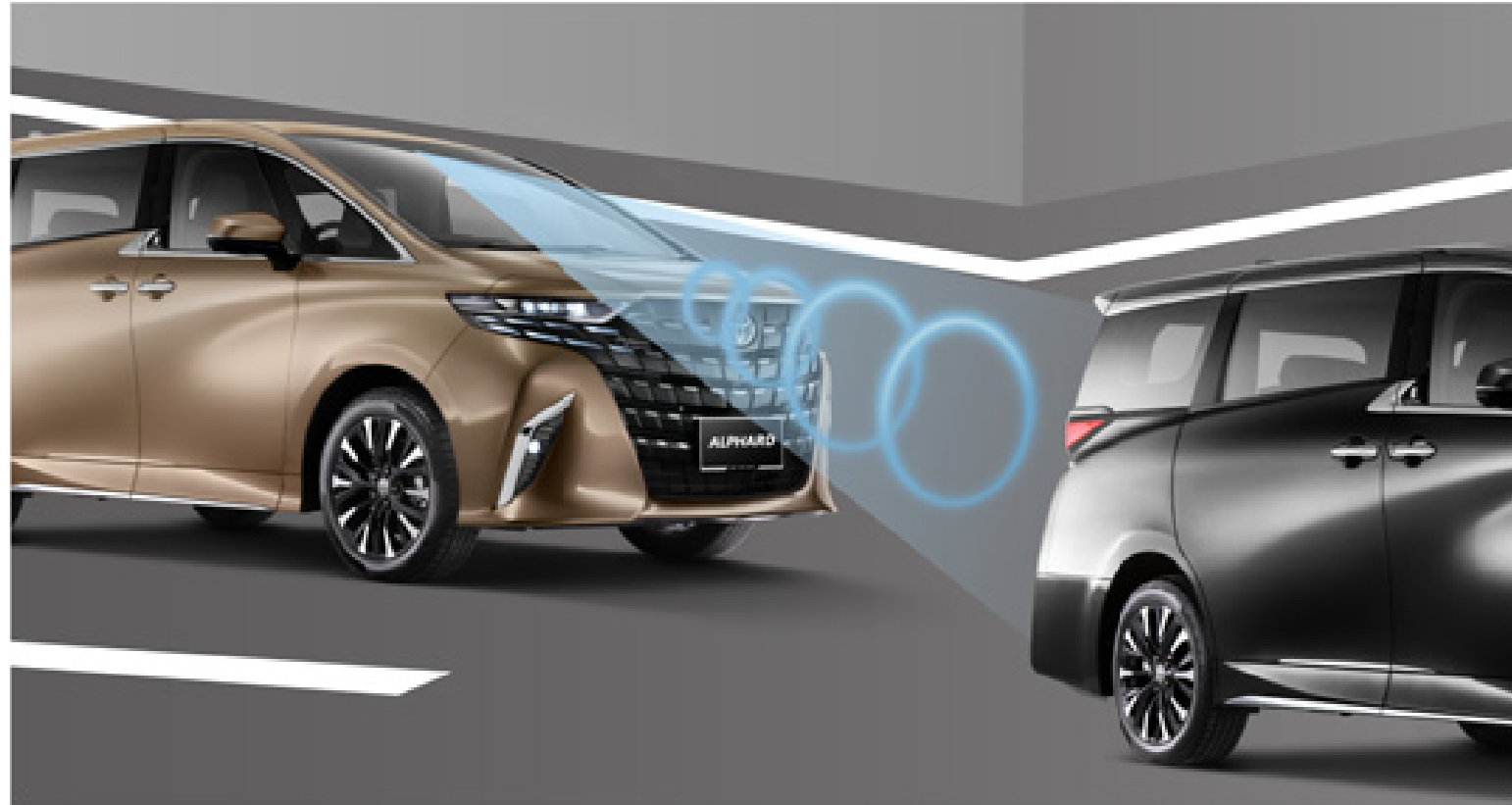
PRE-COLLISION SYSTEM (PCS) Avoids or mitigates frontal collisions by alerting the driver and automatically applying the brakes when there is a risk of collision.
